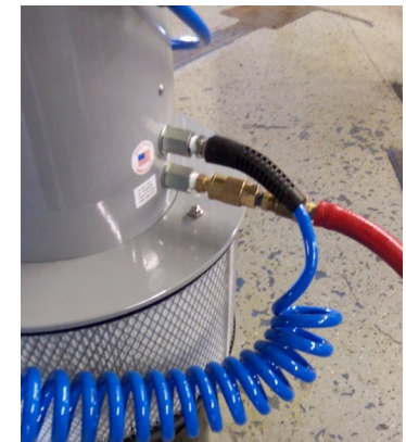
Straight hose supplies the MiJET with compressed air.
